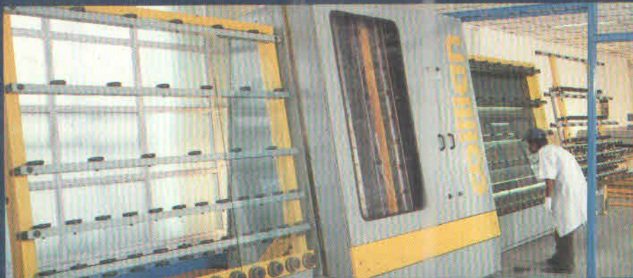
Automatic Insulating Line
